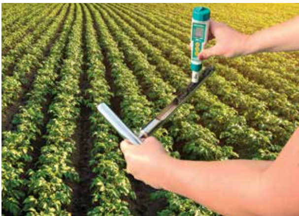
SoilStik shown in use with Item 6510 Model HC Soil Sampler (available online)
