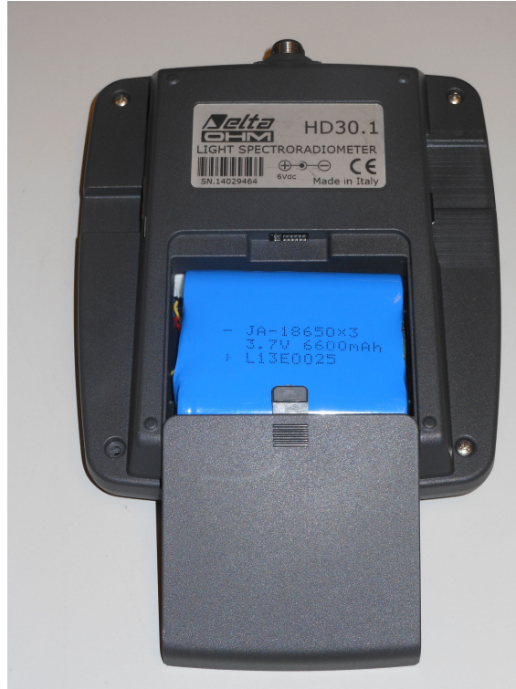
Figure 2.1: Disconnected battery inside battery compartment.
